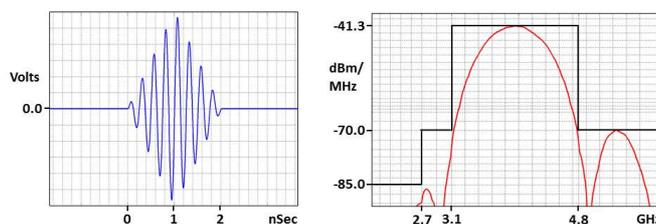
Fig. 2. Nominal pulse in frequency (l) and time domains (r) for EU low band.
