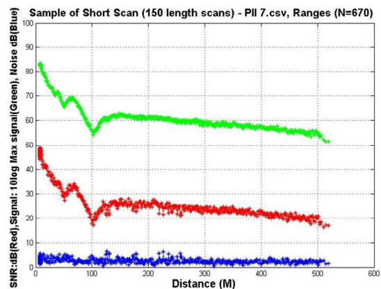
Fig. 6. Sample code allows plotting of range vs Signal strength, SNR and noise.
