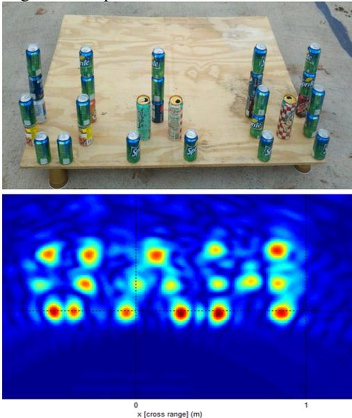
Fig. 10. SAR images of an array of soda cans
