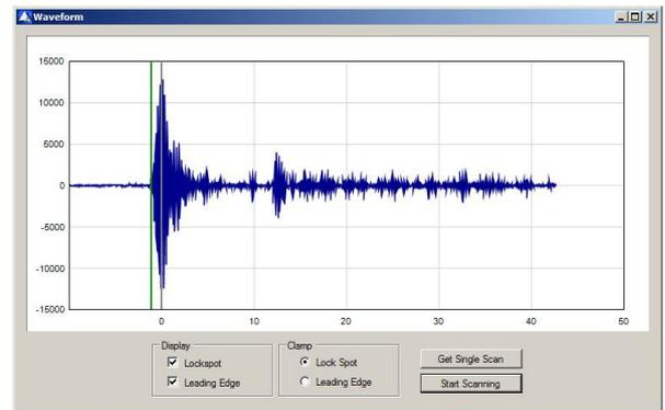
Fig. 3. GUI screen capture illustrating typical channel impulse response/bi-static radar scan.
