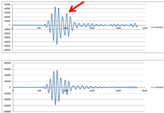
Fig. 5. Response on air (top) vs. over cables (bottom). Arrow indicates likely multipath reflection. (Scale is relative signal strength vs. time in increments of 61ps.)
