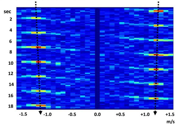
Fig. 11. Doppler processing of radar return of a pendulum in motion.
